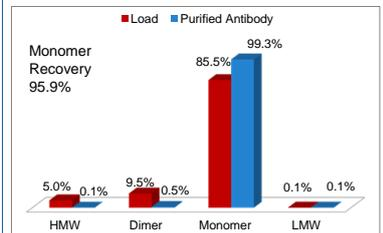
Figure 10. Customer Flow-Through Example for mAb Polish Resin: POROS Benzyl Ultra, Buffer: sodium citrate with a conductivity of 1.7 mS/cm. Flow rate: 500 cm/hr; Product residence time: 1.2 minutes; mAb load: 80 g/L.
